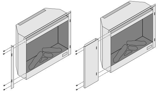
2 The top panel has joggles on the back of the panel that slide over the flanges on the fireplace and panels (see illustration below). Attach the top panel, making sure the ends are square with the side panels.
