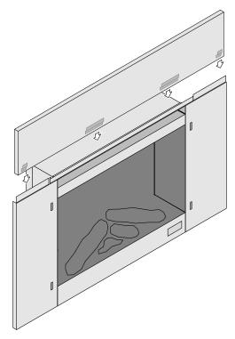
3 Slide the fireplace into position. The side panels have an angled snipe at each bottom corner to allow the power cord to exit the side panels.
