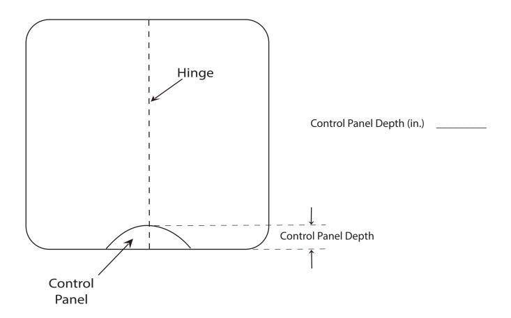
If the orientation of the Smartop on the spa requires the hinge to intersect the control panel acrylic indentation, the depth of the control panel acrylic indentation must be identified so that the wedge can be properly installed for a proper seal with the acrylic of the spa.
